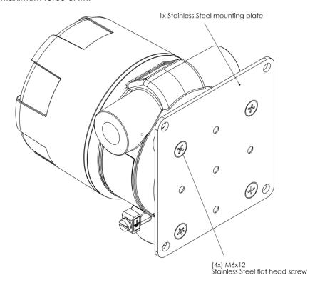
4. Place the mounting plate with the screws to the wall.
