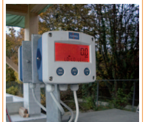
F173 Level Monitor with low alarm
